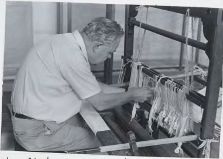
Harold threading up the small loom that will be used for demonstration.
